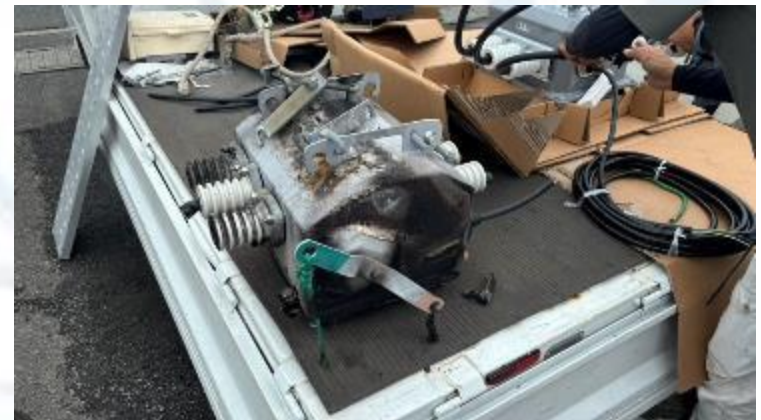
[Switching device burnt by a lightning strike]
