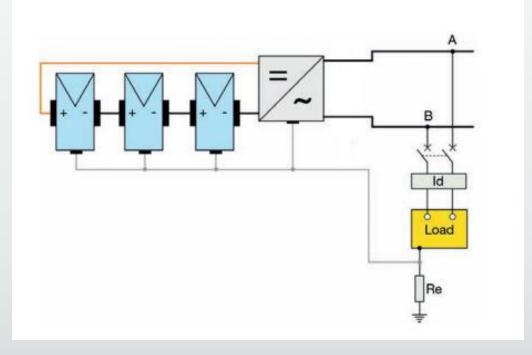
Only metallic frames are earthed and the live parts are Isolated Residual circuit breaker on AC side must be of type B to detect the DC leakage current. However some types of solar panels will be subject to corrosion and degradation due to leakage current which requires the functional earthing of the PV which can only be implemented with galvanic isolation
