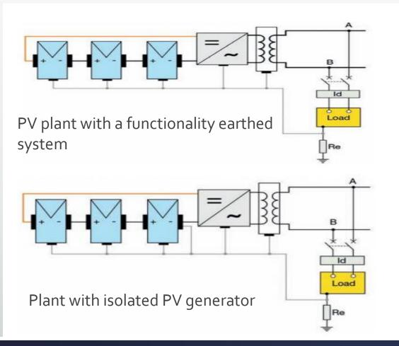
Metallic frame always earthed In case of isolated earthing an Insulation Monitoring Device detects the first fault and trigger an alarm as the second fault will cause a short circuit. NEC code mendates the use of Arc Fault Detection to protect from fire and explosion
