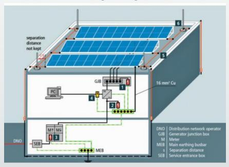
Air termination rod connected to the mesh or ring earthing via down conductor to inject the lightning into earth. Height and separation distance calculated by the rolling sphere method or angle method
