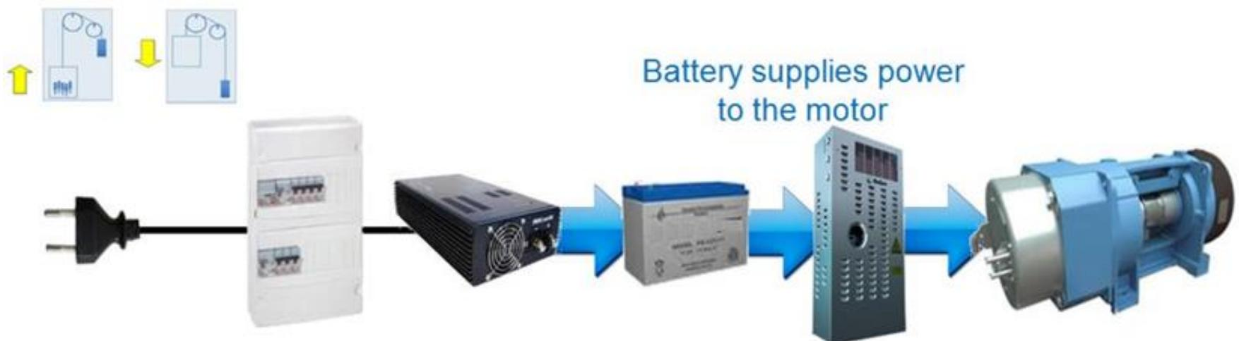
In the normal mode, the battery supplies power to the motor through the ReGen Drive.
