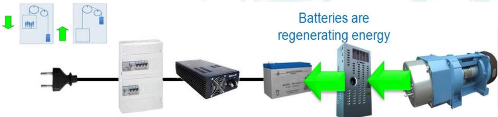
When batteries are full, the energy is consumed in breaking resistance.
