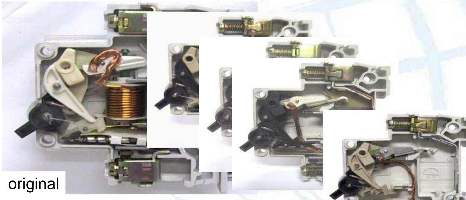
The part that are commonly being removed is the copper coil
